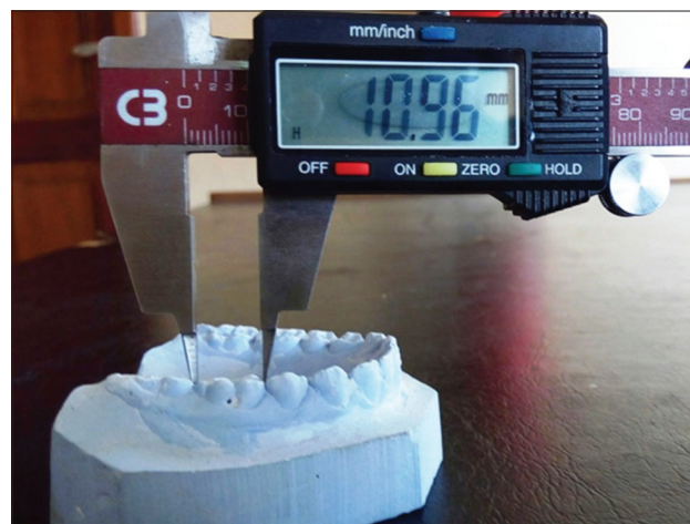
Figure 1: Orientation of the digital calliper for measurements
